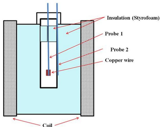
**Fig. 2 Schematic of the cross-sectional view of the quasi-adiabatic calorimetric system used for temperature measurements. Two fiber optic temperature probes are shown in the figure. Probe1 is suspended inside the test tube using a Styrofoam (insulation) secured at the top of the tube, while probe 2 is placed at the intersection of surrounding insulation and the 5 ml polystyrene tube.**
