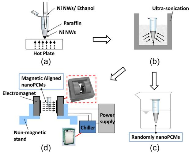
**Fig. 3 Schematic of nanoPCMs preparation process: (a) adding the NWs suspension into melted paraffin. (b) Ultrasonication of the mixture at 80 °C to obtain a uniform distribution of fillers. (c) Rapid solidification in water for randomly distributed NWs in PCMs. (d) Applying magnetic field to obtain align NWs in PCMs.**
