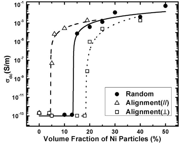
Fig. 6 Dependence of the DC conductivity ( $\sigma_{dc}$ ) on the NPs volume fraction in paraffin matrix at 25 °C for random Ni NPs/paraffin system ( $\bullet$ ), and for magnetic aligned Ni NPs/paraffin system in parallel direction ( $\triangleleft$ ), and in perpendicular direction ( $\square$ ). The lines correspond to the best linear fitting.
