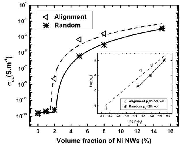
Fig. 7 Dependence of the DC conductivity ( $\sigma_{dc}$ ) on the nickel NWs volume fraction in paraffin matrix at 25 °C for random Ni NWs/paraffin system ( $\ast$ ), and for magnetic aligned Ni NWs/paraffin system ( $\triangleleft$ ). The inset shows the log-log plot of  $\sigma_{dc}$  versus  $(p - p_c)$ . For the random Ni NWs/paraffin,  $p_c = 2\%$ . For the magnetic aligned Ni NWs/paraffin,  $p_c = 1\%$ . The lines correspond to the best linear fitting.
