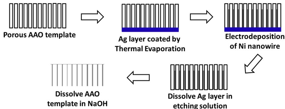
Fig. 1 Schematic of NW synthesis process
