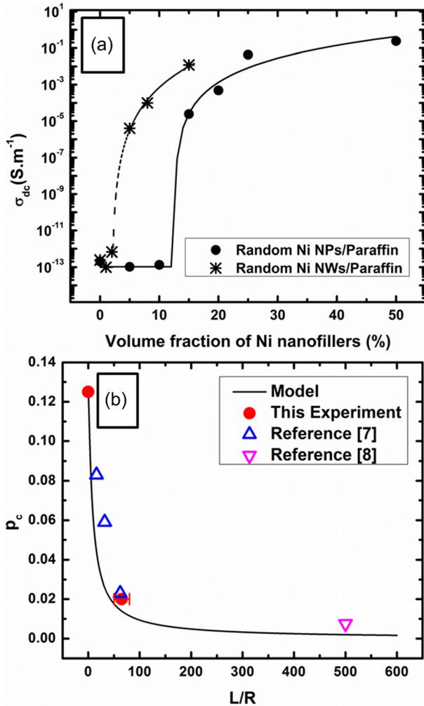
Fig. 5 (a) Dependence of the DC conductivity ( $\sigma_{dc}$ ) on the nickel nanofiller volume fraction in paraffin matrix at 25 °C. (b)  $p_c$  versus  $L/R$  from experiments and the excluded volume analytical model.
