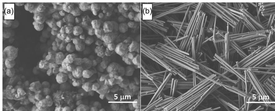
Fig. 2 SEM images of (a) NPs and (b) nickel NWs
