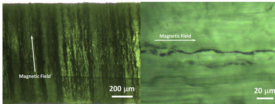
**Fig. 4 Optical microscopic images of magnetic aligned NWs PCM sample with 0.1 vol. % volume ratio (magnetic direction is shown by arrows)**
